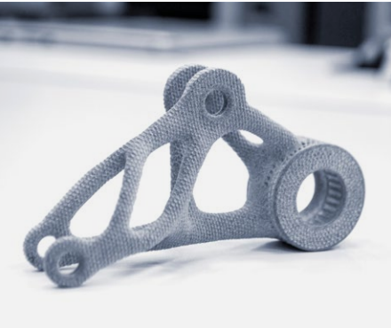
Multi Jet Fusion (MJF): Printing with polymer powder and binding agent.
