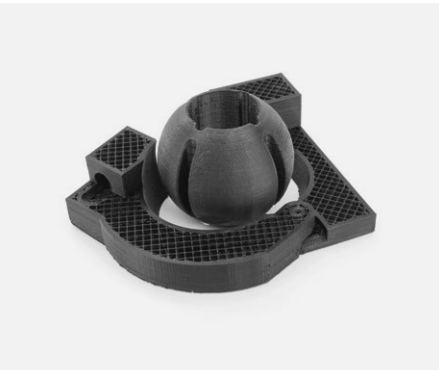
Fused Deposition Modeling (FDM): Printing with plastic filament.
