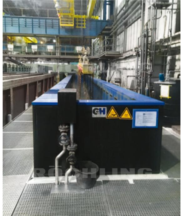
**Exterior cladding made from Polystone® G blue B 100-RC:** The material is suitable for permanent contact with aggressive nitric and hydrofluoric acids and contributes to the plant's high operational safety and performance
